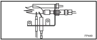
Fig. 17 Correct pilot flame pattern.
